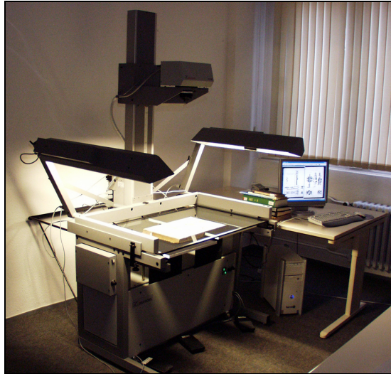
Figure 8. Workstation with a commercial book scanner for digitalization printed media sources
